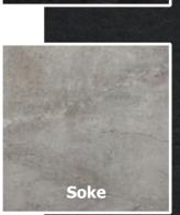
Dekton® is a ceramic material composed of over 20 natural minerals. Compressed under extremely high pressure, it achieves an exceptionally high density and near-zero porosity, making it an ideal choice for worktops, especially in outdoor settings.
